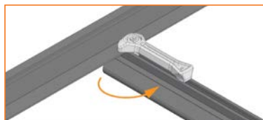
Fig. 4e: CAMO hidden end clamp. Clamp slide into rail channel and the bonding pins contacts the module flange edge.
